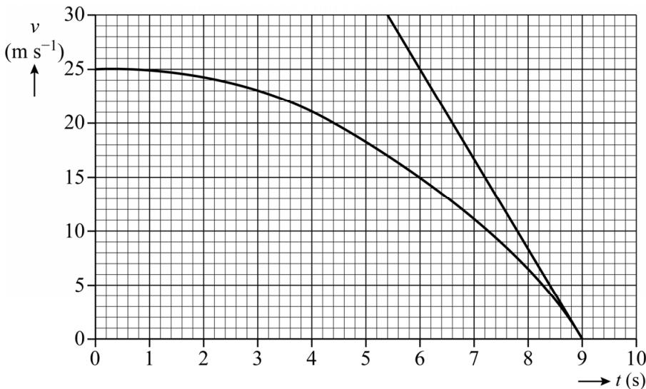
$$\text{Hieruit volgt: } a = \left( \frac{\Delta v}{\Delta t} \right)_{\text{raaklijn}} = \frac{30,0 - 0}{9,0 - 5,4} = 8,3 \text{ m s}^{-2}.$$
